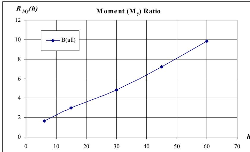
Fig 13. Case (3):Moment (My) Ratio - Shear Wall
